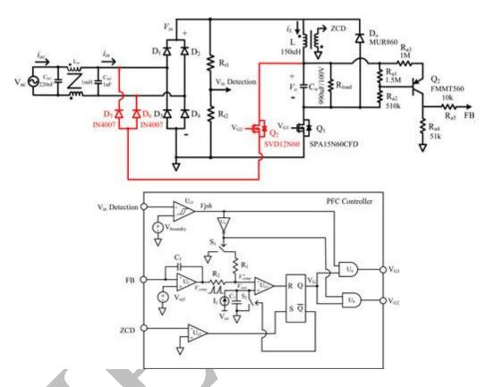
Fig. 5. Schematic of the proposed buck PFC converter with an improved COT control.
