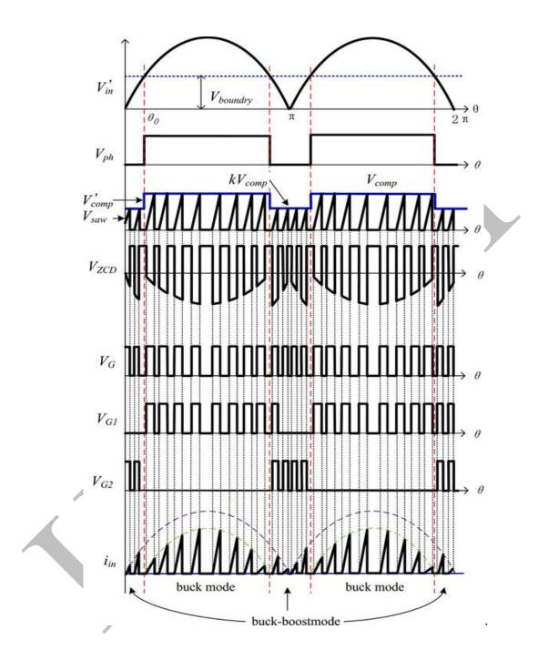
Fig. 6. Key waveforms of rms in the improved COT control diagram.
