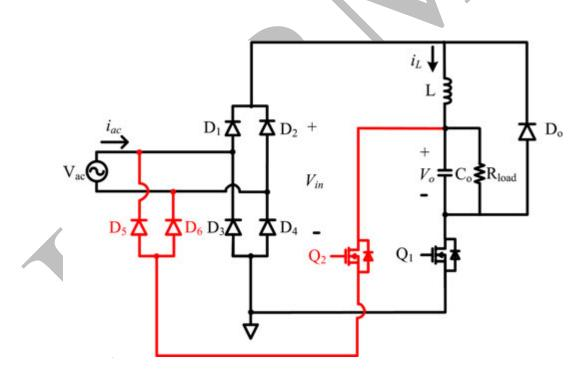
Fig. 3. Improved buck PFC converter.
